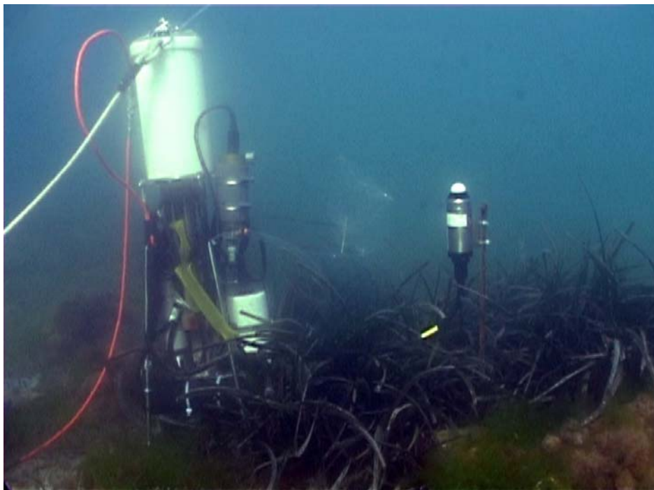
Fig. 4: Benthic chamber and fine scale microprofiler
